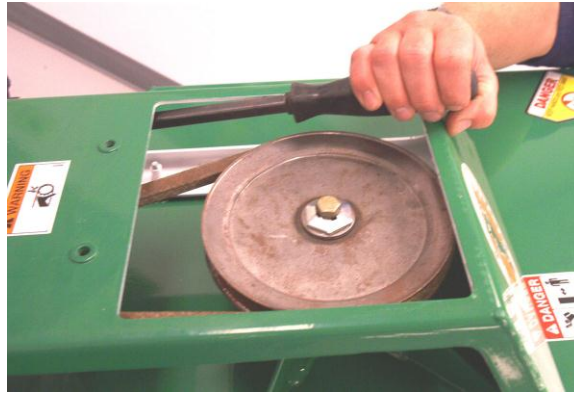
Adjusting Blade Drive Belt Tension
